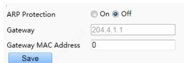
(2) Select the check box to enable the ARP binding function and set the gateway MAC address.
