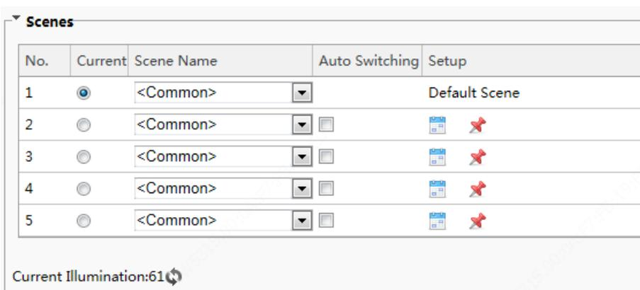
(2) Scene Name: name of the current scene. Several scene modes have been preset in the device. After a scene mode is selected, image parameters are automatically switched (you can adjust image parameters as required).
